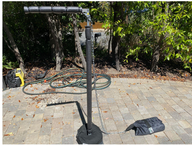
Example of Inadequate Chain Tension:
