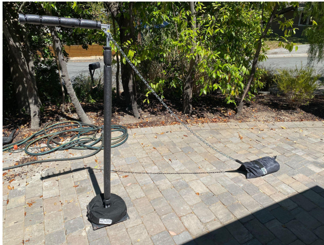
Example of Too Much Chain Tension:
